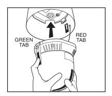
c. Line up the green and red tabs with the green and red labels. Push in on the tabs. Insert the side with the green tab, then the side with red tab. Continue pushing on the ends of the tabs until both sides click into place.
